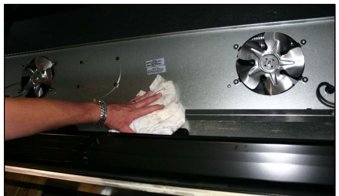
Image #2 Clean under air return grille and fan shroud area with moist cloth. Remove drain cleaning access door and clean drain.
